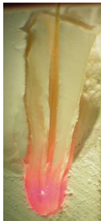
Figure 3. Visible red laser light emitted from an optical fibre with a special surface modification projects 360 degrees in a spherical pattern from the end of the fibre, allowing detection of bacteria in a lateral direction.
