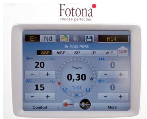
Fig. 5: Touch screen panel showing the PIPST TM setting, at 20 mJ, 15 Hz, no air / no water, 50 microsecond pulse duration.
