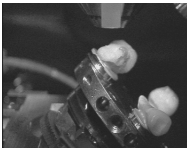
Fig 8: SEM sample chamber.
