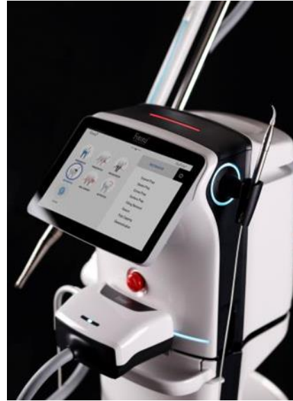
Fig. 4: The SkyPulse Er:YAG laser system used in the study. The laser system is equipped with the two latest laser-assisted irrigation modalities: SSP and SWEEPS, thus enabling a complete SSP/SWEEPS endodontic treatment.
